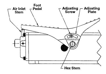
6. Tighten the "Adjusting Screw". The release mechanism is now properly set.
